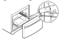
Lower the door into final position and tighten the screws (3) located on both sides.
